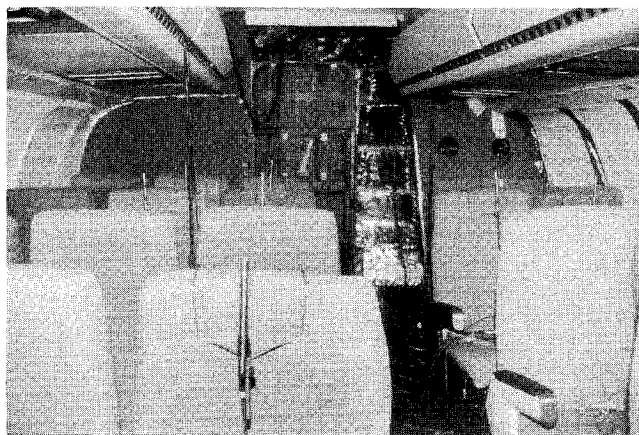
Fig. 2b Cabin interior, facing aft, showing placement of microphones.
